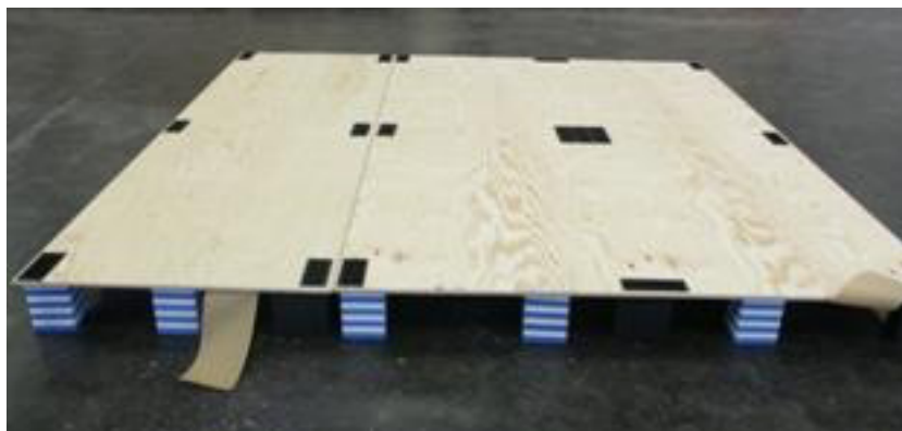
Pic. 6: Plywood sections with mounted foam cubes and velcro tape
