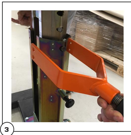
4. Check the Ergojet Rio version by looking to the axis on the outer column. Is there a small hole and which handle does your Ergojet have?
