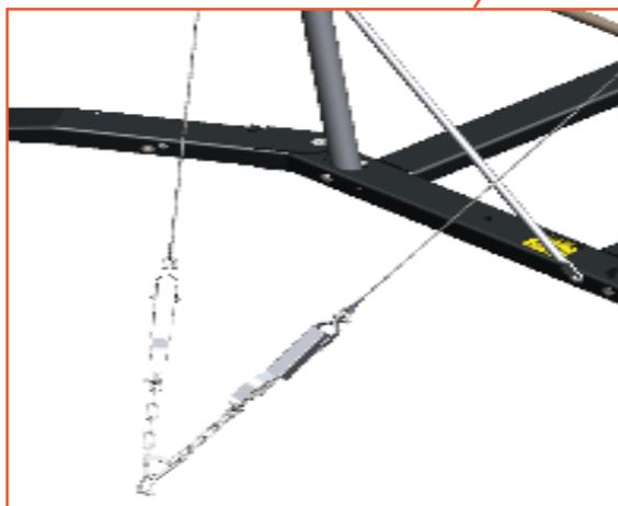
2. Attach the tensioning back left to the ground anchor (Pic. 10)
